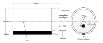
Solder Pin Type 4 pin 300F, 400F Part
