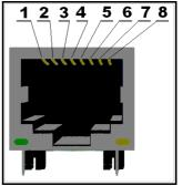
The two leds on the front side of the LAN connector show the state of the Ethernet. The meaning behind the different states can be found in the table below:
