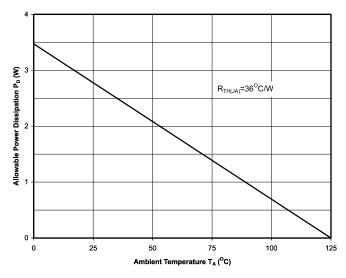
Figure 1. Power Derating Curve
