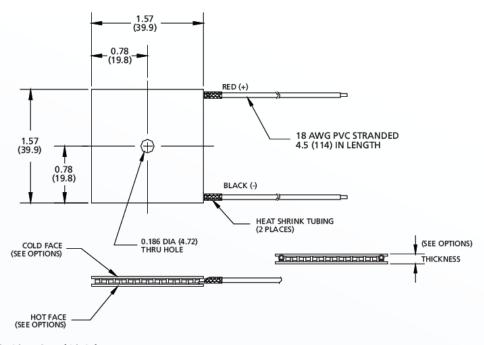
Ceramic Material: Alumina (Al<sub>2</sub>O<sub>3</sub>)
