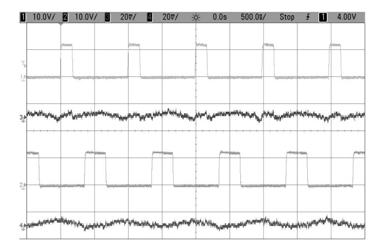
Figure 3. LTC3633A-3 DC1896 Switch Operation
