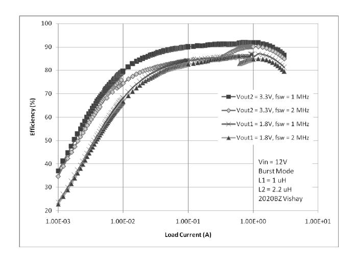
Figure 6. LTC3633A-3 DC1896 Efficiency
