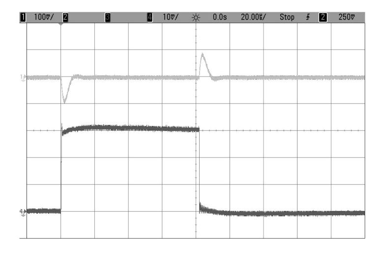
Figure 4.  $V_{OUT1}$  Load Step Response
