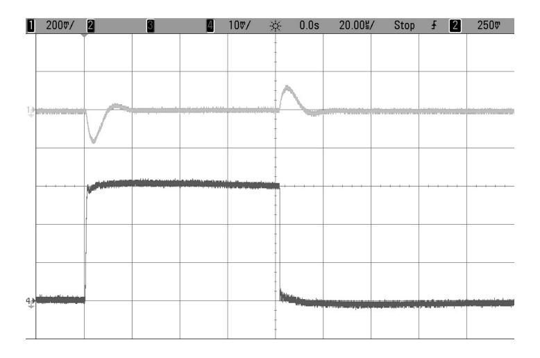
Figure 5. V<sub>OUT2</sub> Load Step Response
