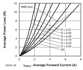
Fig. 6 - Forward Power Loss Characteristics
