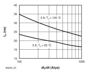
Fig. 7 - Typical Reverse Recovery Time vs. dl<sub>F</sub>/dt
