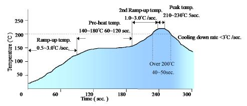
Note: The temperature refers to the pin of V48SC, measured on the +Vout pin joint.
