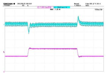
**Figure 8:** Output voltage response to step-change in load current (50%-75%-50% of full load; di/dt =  $0.1A/\mu$ s). Load cap:  $10\mu$ F, tantalum capacitor and  $1\mu$ F ceramic capacitor. Top Trace: Vout; 50mV/div; Bottom Trace: output current: 5A/div, Time: 100us/div
