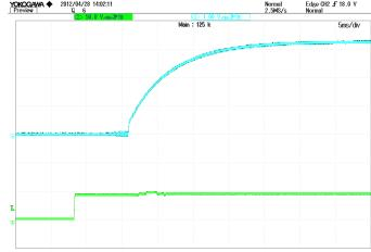
**Figure 6:** Turn-on transient at zero load current (5 ms/div). Top Trace: Vout; 1V/div; Bottom Trace: input voltage: 50V/div.
