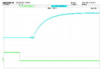
**Figure 4:** Turn-on transient at zero load current) (5ms/div). Top Trace: Vout; 1V/div; Bottom Trace: ON/OFF input: 5V/div.
