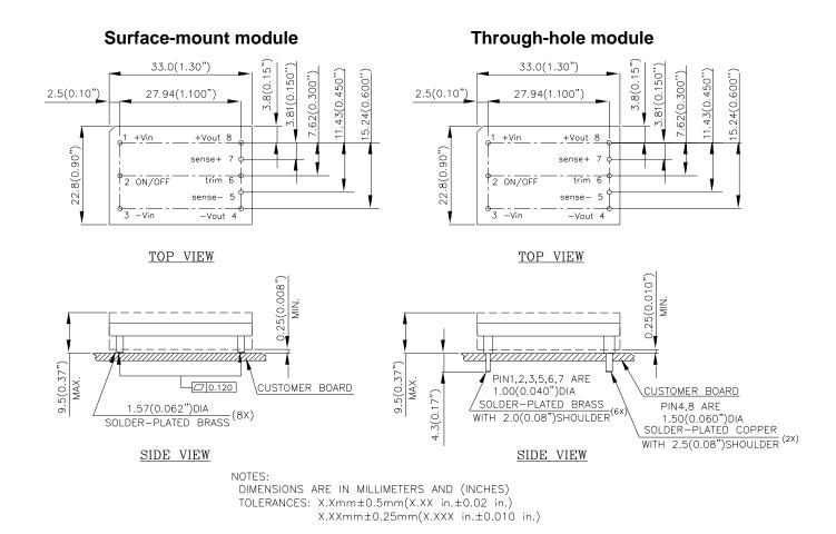
Note: All pins are copper alloy with matte Tin(Pb free) plated over Nickel under plating.
