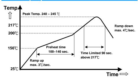
Note: The temperature refers to the pin of V48SC, measured on the +Vout pin joint.
