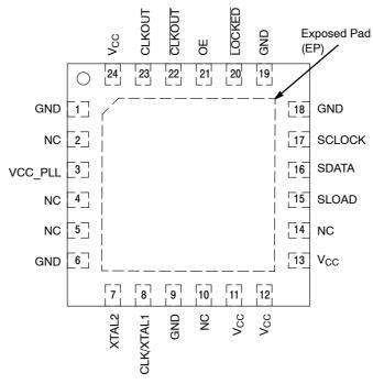
Figure 3. QFN-24 Lead Pinout (Top View)
