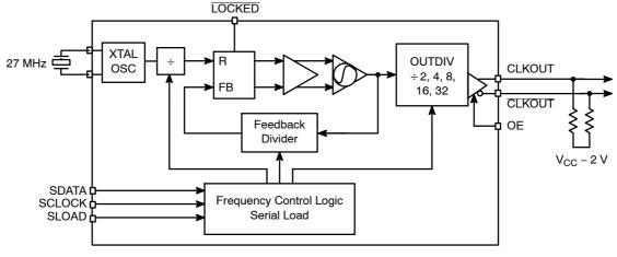
Figure 1. Simplified Block Diagram
