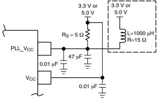
Figure 4. Power Supply Filter
