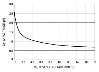
Figure 3. Typical Capacitance
