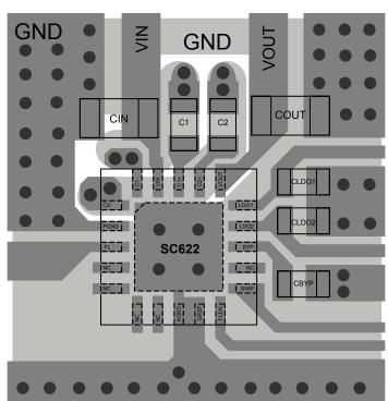
Figure 1 — Recommended PCB Layout
