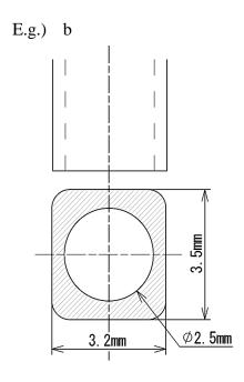
\*Nozzle with chamfering is recommended
