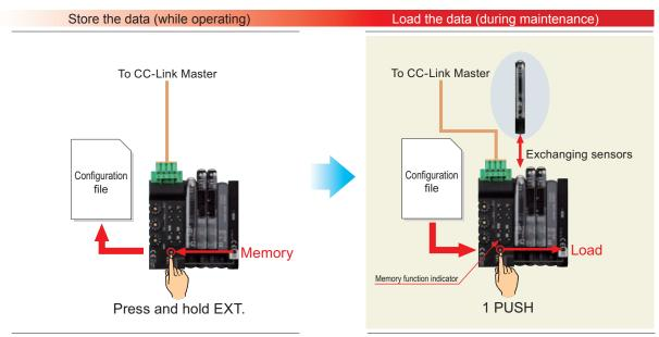
\* Memory function can be utilized with CC-Link communication by setting the flag in the remote register.
