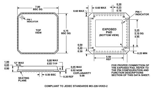
Figure 5. 48-Lead Lead Frame Chip Scale Package [LFCSP\_VQ] 7 mm × 7 mm Body, Very Thin Quad (CP-48-1) Dimensions shown in millimeters
