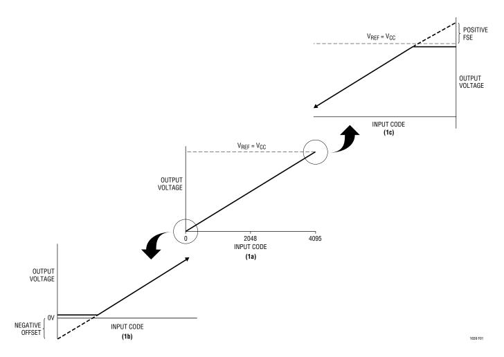
Figure 1. Effects of Rail-to-Rail Operation on a DAC Transfer Curve
